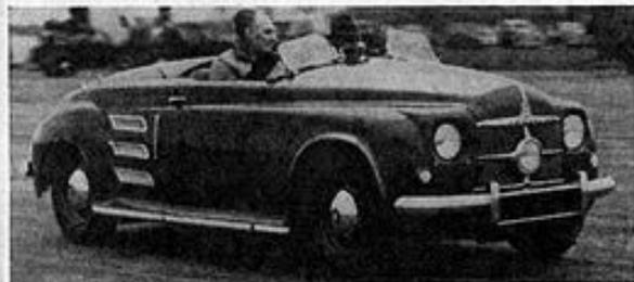
Twin kerosene-fed jet turbines propel this British Rover Motor Co. turbine-powered car. Driver uses only two pedals—accelerator and brake.
