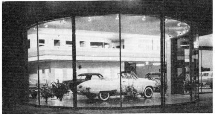
SEMI-CIRCULAR SHOWROOM section, featuring a floor-flush turntable on which a car makes a complete turn of the 18-foot diameter circle every 100 seconds, is the outstanding feature of the quarter-million-dollar new building of Stewart Motor Co. (Studebaker) just opened in Phoenix, Ariz.
