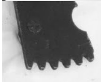
New false teeth from good part of regulator
