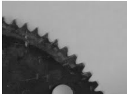
New false teeth welded into place
